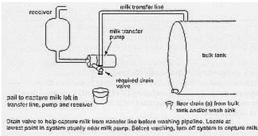
Prerinsing can also be programmed into some clean-in-place systems, and a diverter valve installed to automatically divert the prerinse to a bucket. Milk collected by prerinsing can be fed to calves or hogs if it is not too watery or contaminated with cleaning chemicals. If it is not used to feed animals, you should deliver the rinsate to manure storage or put it in a manure spreader.
