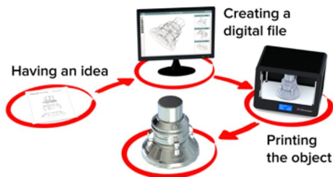
**Material extrusion** is one type of 3D printing, and it is the most common one for use at home. This process is also sometimes called **fused deposition modeling (FDM)** or **fused filament fabrication (FFF)**. This process builds parts using plastic material.
